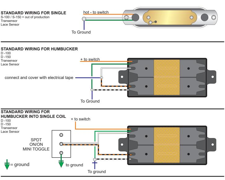
The Lace Sensor Dually can be Split into single top / both /single bottom by using a SPDT on/off/on Mini Toggle Switch.
